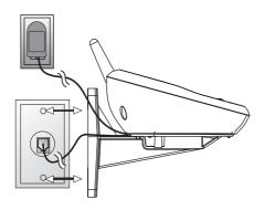
4. Line up the tabs on the wall mount bracket with the slots on the bottom of the base unit. Snap the bracket firmly in place.
